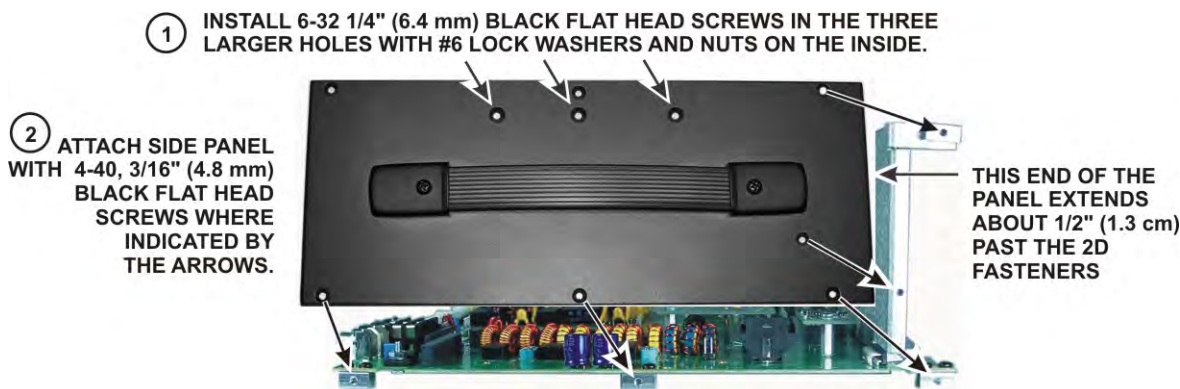
Figure 16. Mounting Left Side Panel.
