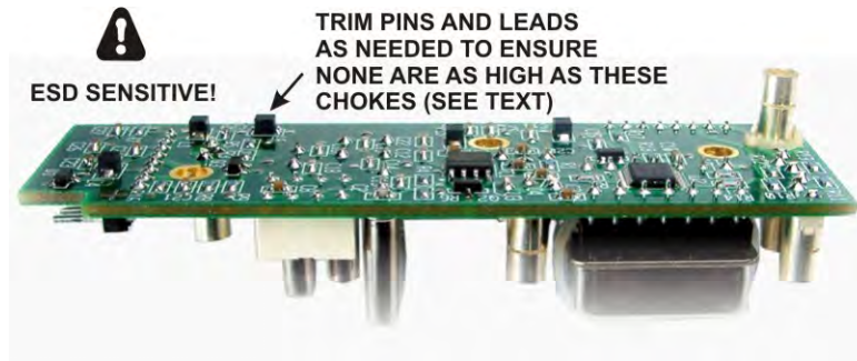
Figure 69. Checking Lead Lengths on KREF3 Board.
