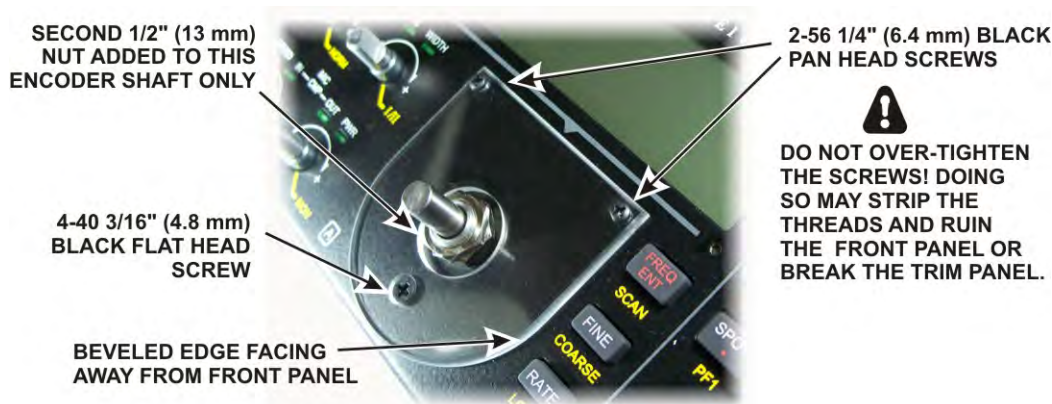
Figure 44. Mounting VFO A Trim Panel.
