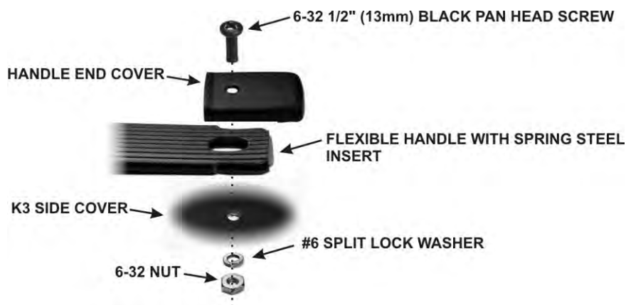
Figure 15. Installing Side Handle Mounting Hardware.
