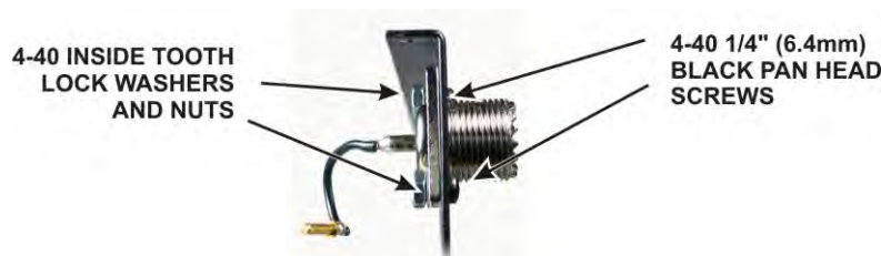
Figure 18. Mounting the ANT1 Connector.
