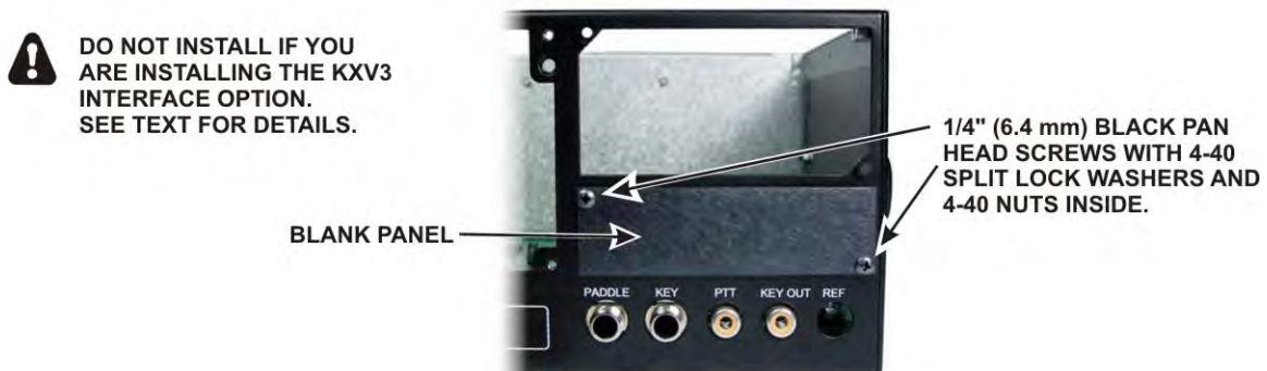
Figure 31. Preparing Rear Panel for KIO3 Installation.
