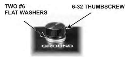
Figure 27. Installing Rear Panel Ground Screw
