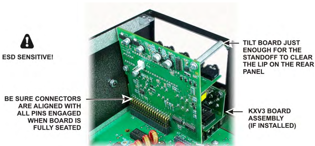
Figure 33. Installing KIO3 Main Board.
