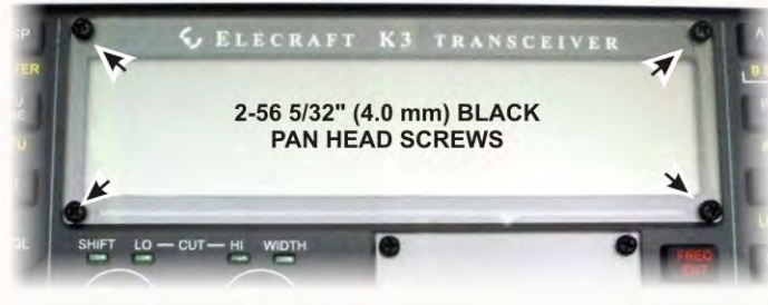
Figure 46. Installing LCD Cover.
