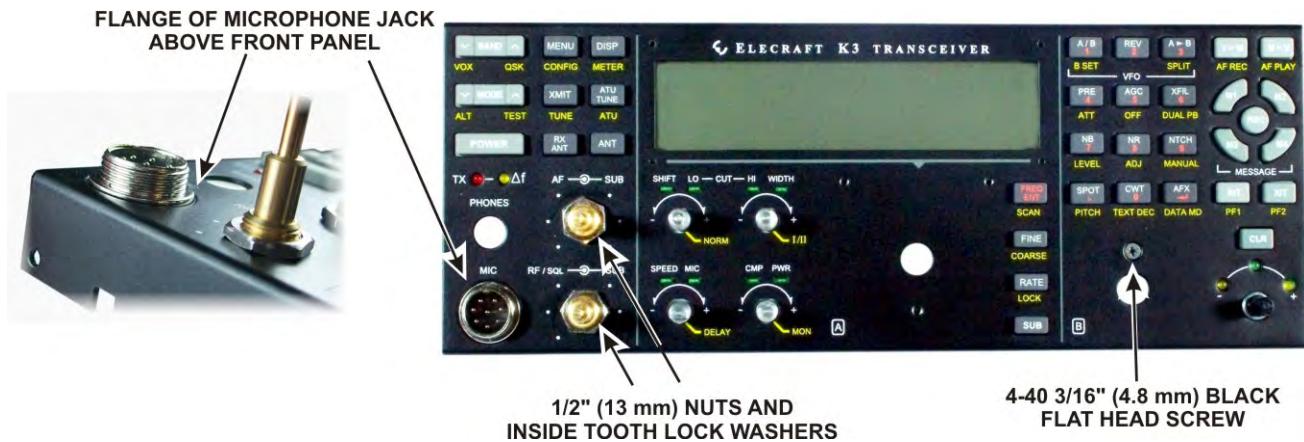
Figure 40. Mounting the Front Panel on the Front Panel Board.
